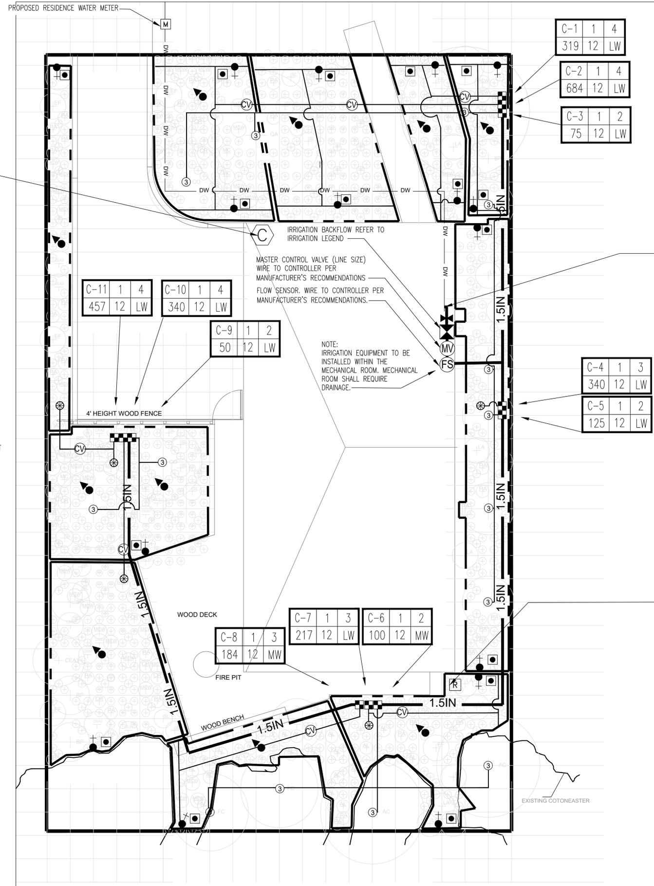
IRRIGATION CONTROLLER "C". MOUNT ON INTERIOR WALL AT THIS LOCATION AS DETAILED AND AS DIRECTED BY ARCHITECT. CONNECT TO 120 VOLT A.C. ELECTRICAL SERVICE INSTALLED AT THIS LOCATION UNDER ELECTRICAL CONTRACT. IRRIGATION CONTRACTOR SHALL COORDINATE LOCATION OF ELECTRICAL SERVICE PRIOR TO CONSTRUCTION.
