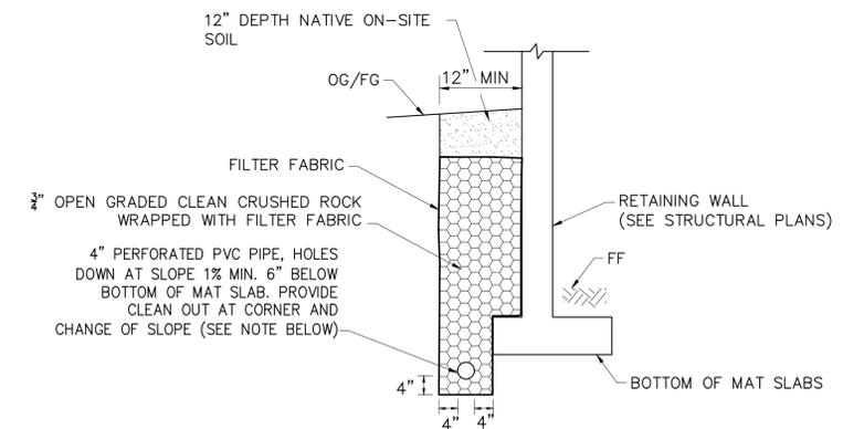
NOTE: ALL PIPING USED SHOULD HAVE COUPLINGS THAT ARE GLUED OR HAVE RUBBER GASKET JOINTS TO ENSURE THAT THE PIPE SECTIONS WILL NOT SEPARATE.
