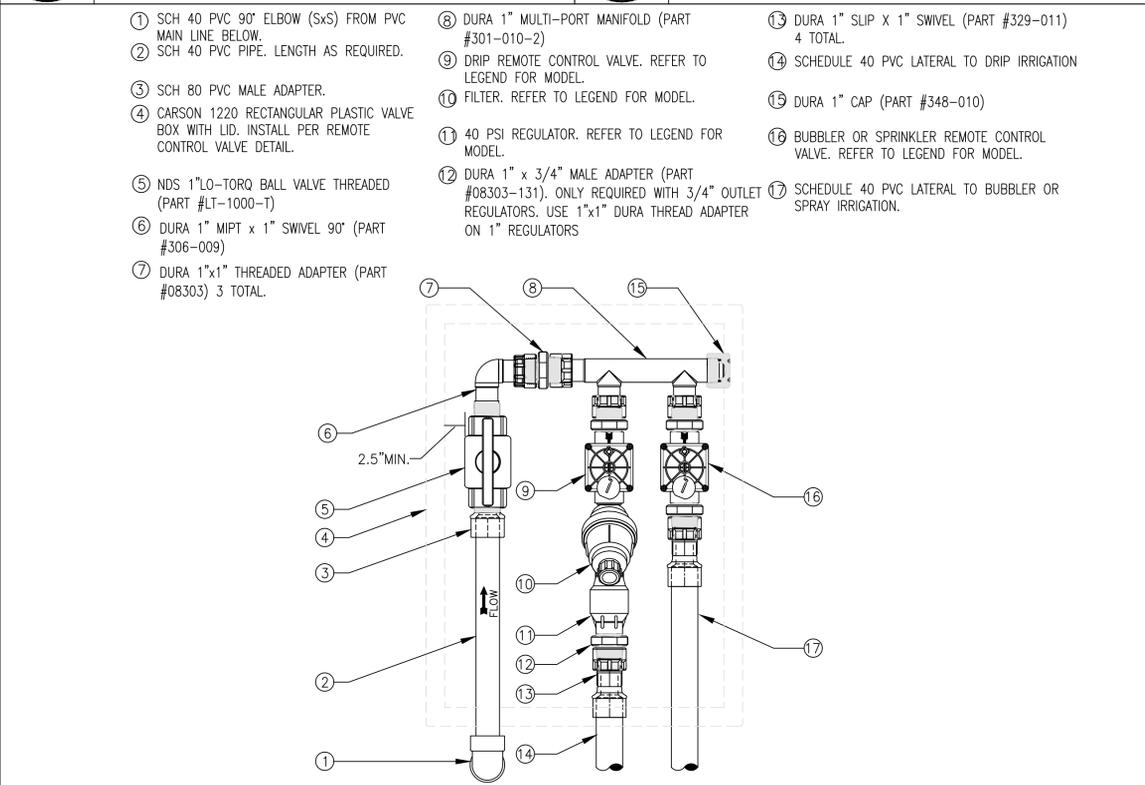
4 TWO REMOTE VALVE MANIFOLD DETAIL
