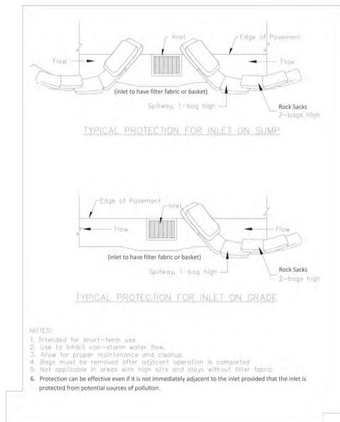
**Storm Drain Inlet Protection SE-10**
